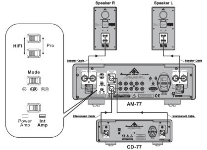
This is the factory default setting: the connection for which has been described in detail in *Section 1 - Unpacking and Setup*. We have illustrated the default switch positions here for ease of reference to re-configure from an alternative system setup back to the pre-main stereo amplifier mode.
